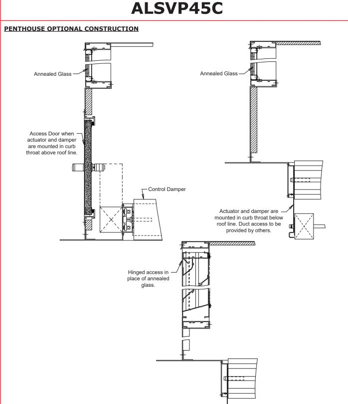
Actuator and damper are mounted in curb throat below roof line. Duct access to be provided by others.
